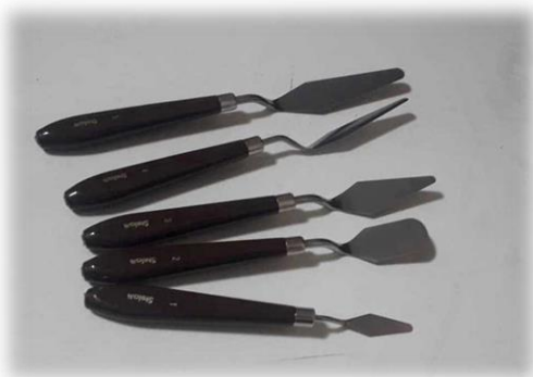
Set of spatulas for applying putty, plaster, white cement etc.
